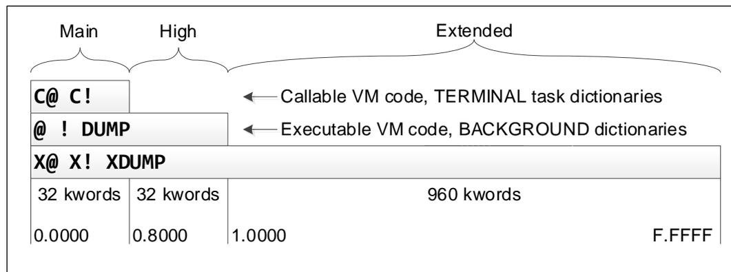
Main memory is allocated by the **OPERATOR** task using the conventional words as follow:
